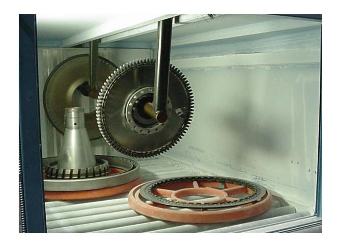
After a drying step, developer is applied, typically using either a spray application or developer chamber as shown here.
