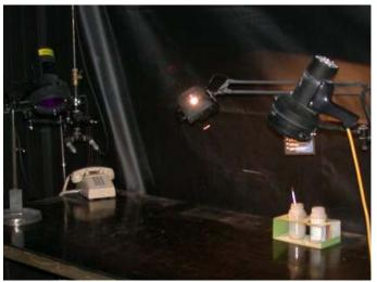
Upon completion of adequate developer dwell time, component is inspected under blacklight in a darkened room or booth
