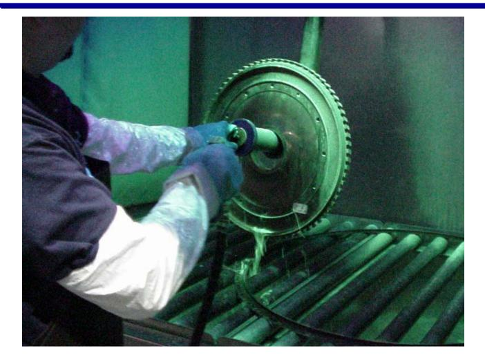
After the specified dwell time, excess penetrant is removed typically using a spray pre-rinse of acceptable temperature and pressure.
